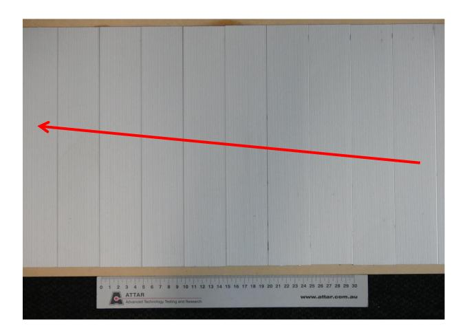
Figure 1: Nexost Stair Nosing and Corrugated insert Arrow indicates direction of testing
